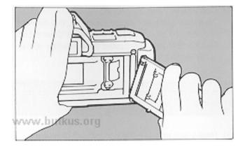
Be sure that there is no film in the camera before attaching the Command Back. Other wise, the film will be exposed when the regular camera back is opened.
