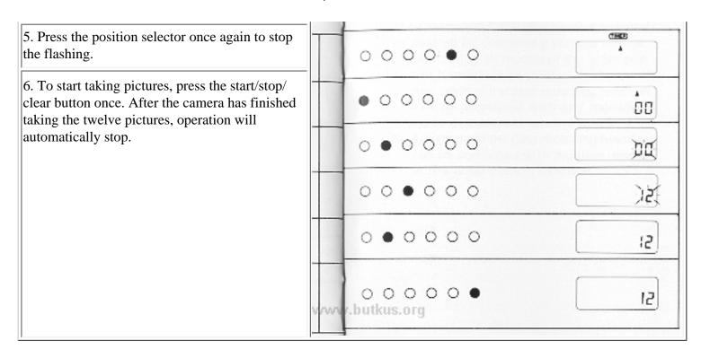
Note: If the frame counter of the Command Back is set to 00, shooting is impossible even when the start/stop/clear button is pressed.
