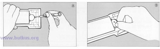
When the " " mark appears to the right of "BATTERY" on the Command Back 70 or 80, the battery has become exhausted. With the Command Back 90, the " " mark will appear to the right of the " " mark. At this time, replace the battery promptly as instructed below.
